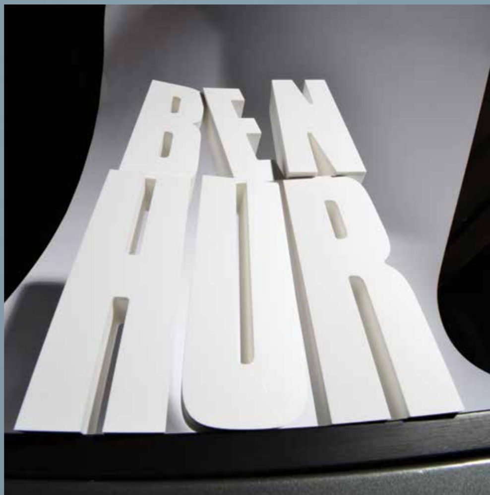
Title letters were laser cut from doubled-up foamex and photographed at an angle to give the illusion of immense height. Also, behind the scenes images.
